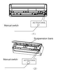
NOTE: The unit must be turned off before operating the manual control button. If the unit is operational, continue pressing the manual control button until the unit off.
